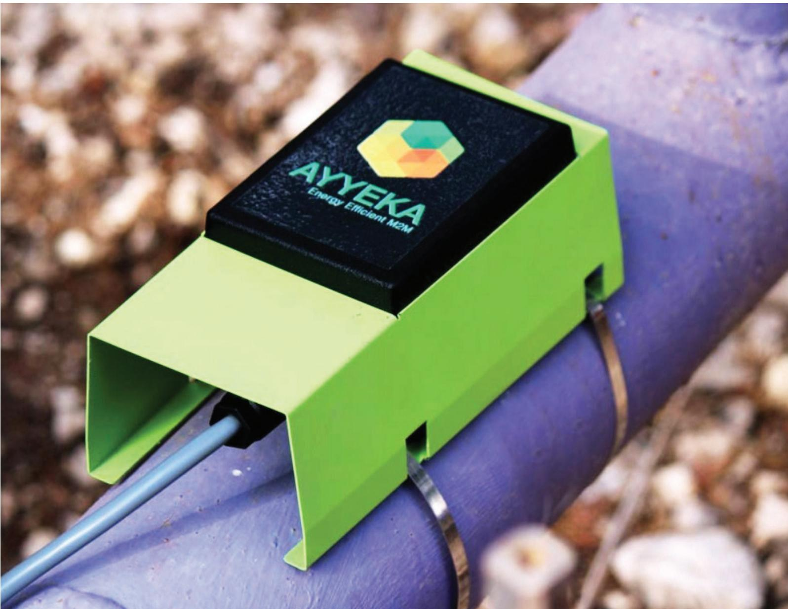
Figure 1: Wavelet Water Quality Kit Installed onto Existing Pipe.
