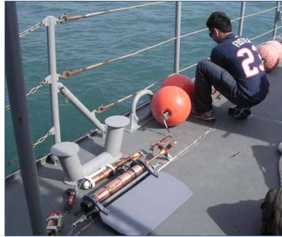
Instrumented oceanographic mooring for the Shamal study, including PME Cyclops-7 fluorometers and PME miniDOT dissolved oxygen sensors.
