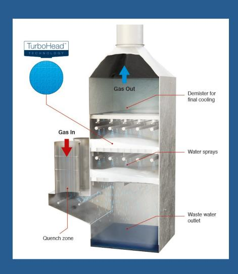
Scrubber water samples from additional run with HGO were also acquired using a wet scrubber system similar to the one depicted in the diagram here
