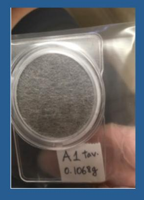
A10 filter membrane is the Sampling Blank from offline filter holder (collecting lab ambient air)
