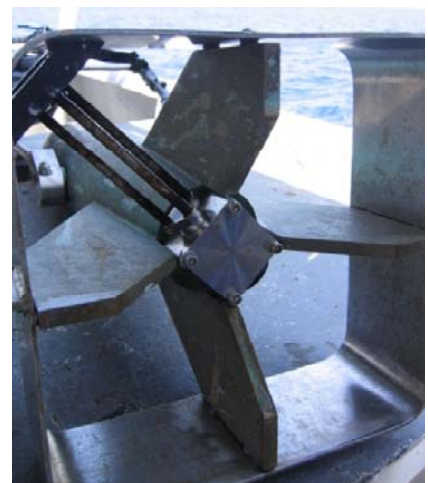
Figure 4. AML SV&P sensor (on single sensor fish)
