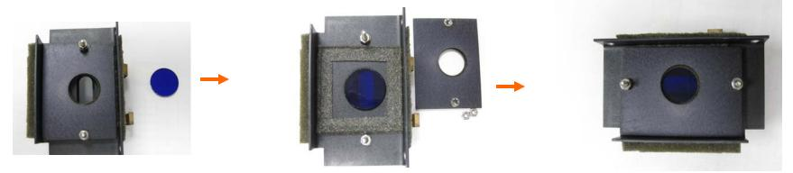
Emission Filter Assembly P/N 1000-260 and Install:
