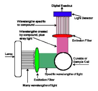
*3.21 Light Source*: The lamp or light source provides the energy that excites the compound of interest by emitting light. Light sources include xenon lamps, high pressure mercury vapor lamps, xenon-mercury arc lamps, <sup>9</sup> lasers, and LED's. Lamps emit a broad range of light; more wavelengths than those required to excite the compound. Lasers and LED's emit more specific wavelengths.
