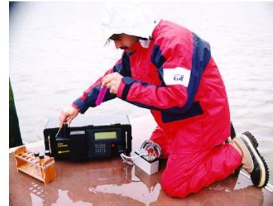
The Model 10-AU Field Fluorometer in use in a fluorescent tracer study.
