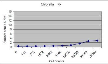
**Figure 9:** *Chlorella* sp.(a green alga containing no phycobilin pigments) sensitivity of the SCUFAfluorometer with phycocyanin optics. The graph indicates that algal groups not containing phycocyanin do not interfere with the fluorescence readings.
