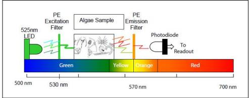
Figure 3: Fluorometer configuration for detection of phycoerythrin
