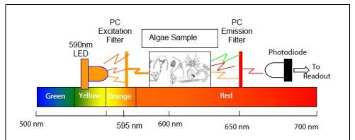
Figure 2: Fluorometer configuration for detection of phycocyanin
