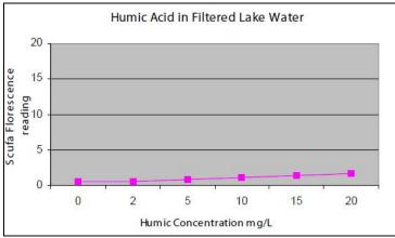
Figure 10: Graph of simulation of natural lake water versus humic interference in optical detection of the SCUFA fluorometer with phycocyanin optics. Even at high humic concentrations there was not a significant fluorescence signal indicating that the optics are not susceptible to humic interference.
