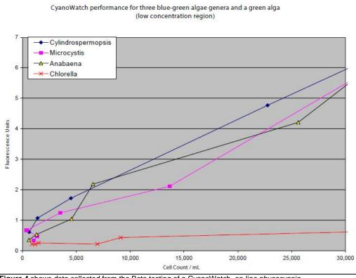
**Figure 4** shows data collected from the Beta testing of a CyanoWatch on-line phycocyanin instrument. Three cultures of phycocyanin containing cyanobacteria were tested and one species of green algae as a control. The data indicates that the instrument detected all three cyanobacteria cultures at low concentrations while the green alga was not detected.
