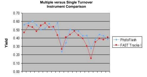
**Figure 3**. Comparison of Turner Designs' PhytoFlash and Chelsea's Fast Tracka I during combined profiles in Monterey Bay. The PhytoFlash was deployed with a shade cap.
