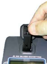
Photo 2. Placing the adjustable secondary standard in the instrument
