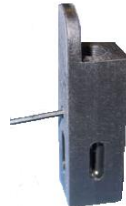
Photo 1. Loosening the locking setscrew on the backside of the adjustable secondary standard
