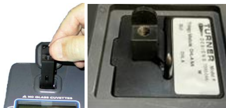
Photo 2. Placing the adjustable secondary standard in the instrument
