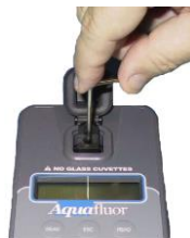
Photo 3. Adjusting the value on the secondary standard by turning the attenuation screw.
