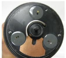
7) Repeat steps 1-6 to apply copper tape pieces to the C3's optical head as pictured below
