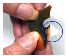
2) Remove the adhesive backing from the other arm of the copper tape piece
