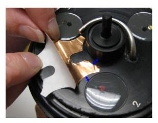
4) Remove the rest of the adhesive backing from the copper tape
