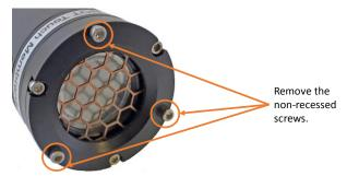
Carefully remove the copper shield faceplate.
