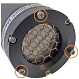
CAUTION: It is important to ensure the copper screen does not contact the stainless steel head cap screws or the sensor membrane as this will result in galvanic corrosion of the head screws. If the Pumped Head Assembly is used the Antifouling Guard can be used but you must install longer screws.
