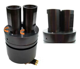
4) Rotate the Solid Standard(s) until set into position. *Note: You will feel/hear a click when the Solid Standard is positioned properly.*
