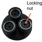
To change the signal level, insert the green screwdriver through the hole in the locking nut. Rotate it in either direction until it engages with the adjustment screw that is beneath the locking nut.
