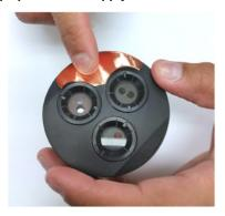
4) If the copper tape is not contacting any of the sensor heads and is within the inner diameter of the Cyclops Integrator's Optical Head, use your finger to apply pressure to all parts of the copper tape to smooth any bumps, rough parts, or detached edges
