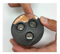
Repeat steps 1-4 to apply copper tape pieces to the Cyclops Integrator's Optical Head as pictured below
