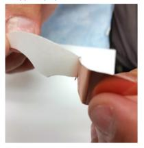
With the adhesive side down, carefully align the copper tape piece on the outside of the sensor heads rings. Make sure the copper tape doesn't contact any of the sensor heads
