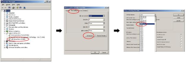
With only the USB cable attached to the computer (do not have it connected to the DataBank), open the Device Manager for Windows and establish which port it is connected to. Select the port and "right click" to open the Properties window. Select the Port Setting tab and select the Advanced button.
