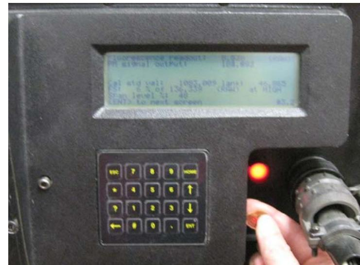
**8. When the %FS reaches the designated value, tighten the sensitivity locking screw.
