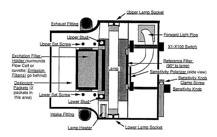
Figure A2. Sample Compartment, Cover Removed
