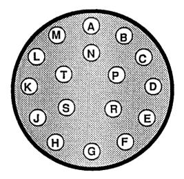
Figure A4. Power/Telemetry Connector Pins
