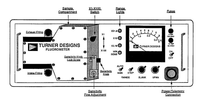
Figure 1. Model 10 Fluorometer Controls & Indicators (shown with Continuous-Flow Cuvette)
