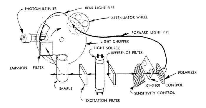
Figure Al. Optical System of the Model 10 Fluorometer
