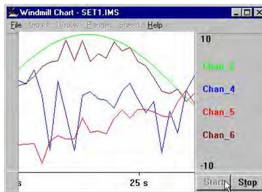
The Windmill Chart window, with data from 4 channels superimposed on 1 axis.
