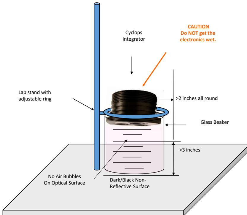
5. Ensure the optical face of the sensor is fully submerged in solution.
