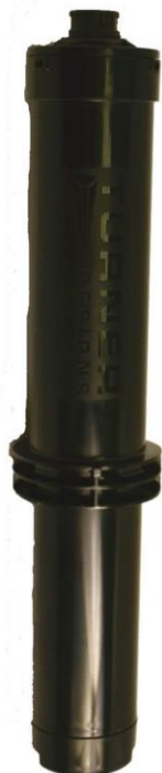
Little Dipper™ 2 Fluorometer with label specifying serial number of unit
