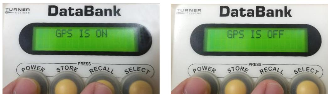
**Note:** *GPS operation impacts battery life, to estimate battery life refer to Section 5.7.*
