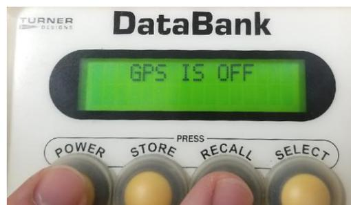
**Note:** *GPS operation impacts battery life, to estimate battery life refer to Section 5.7.*
