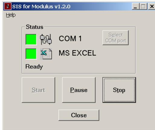
Spreadsheet Interface Software status window example showing communications are set up on COM 1 and that the data will be displayed in an EXCEL spreadsheet
