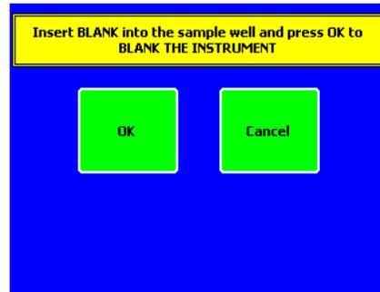
d) When the blanking is complete, the display will revert to the Absorbance Home/Measurement Screen.
