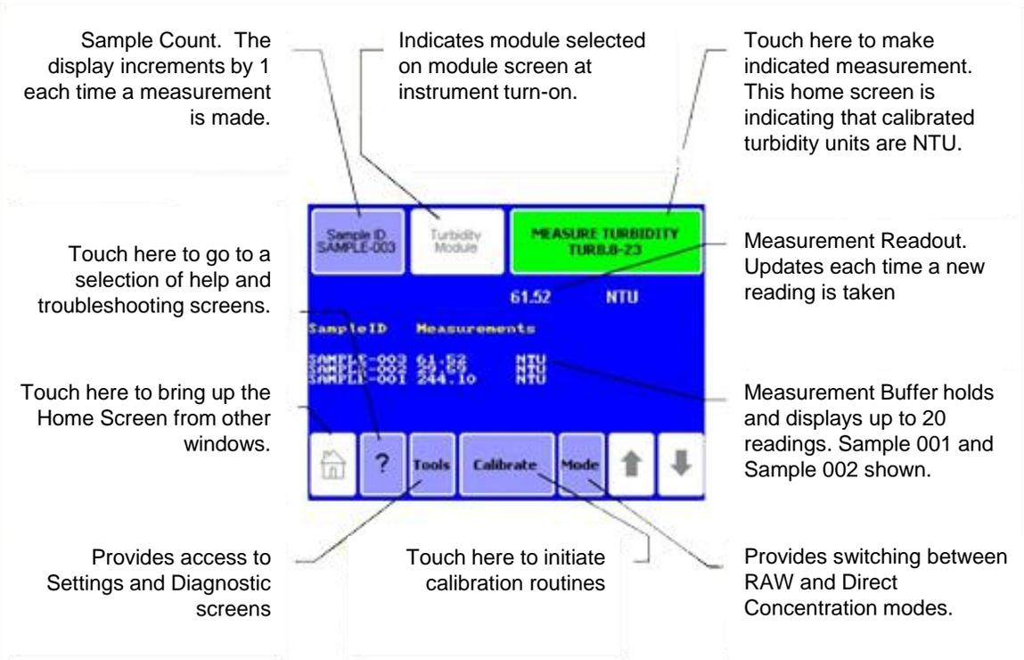
**Figure 7:** Home Screen When Using Turbidity Module
