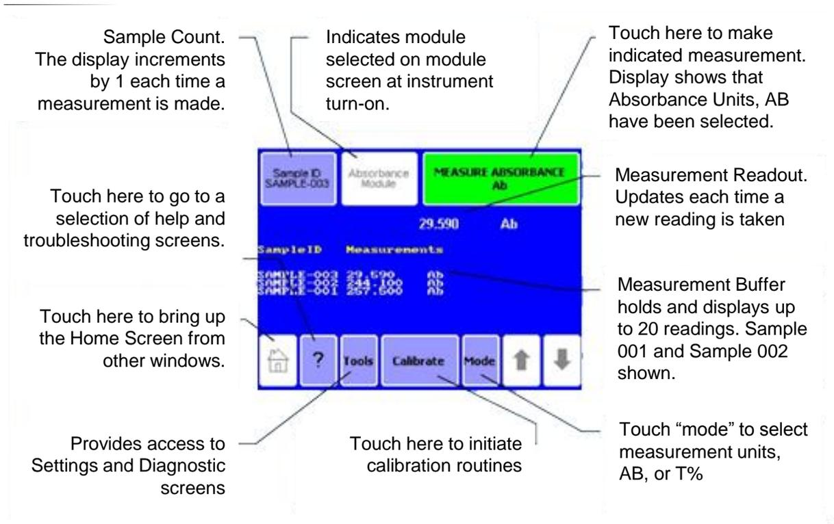
**Figure 6:** Home Screen When Using Absorbance Module
