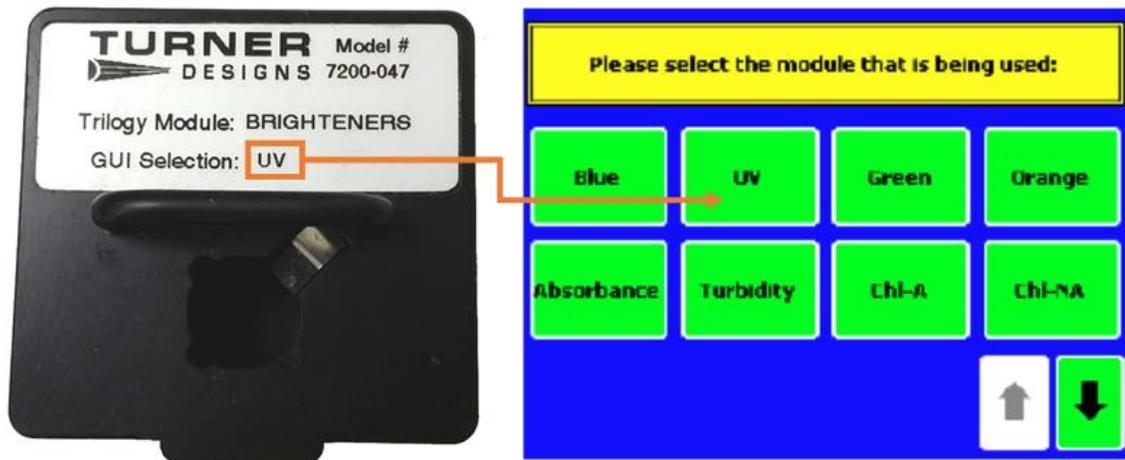
3. Select the module inserted and touch **“OK”** on the confirming screen.
