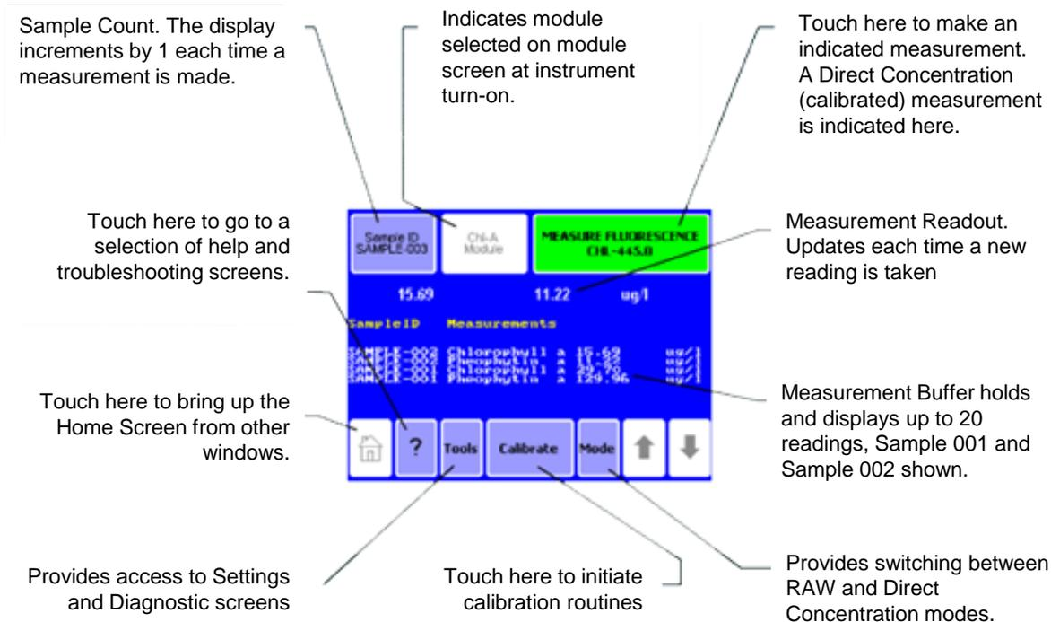
**Figure 4:** Trilogy Home Screen Display for Fluorescence Module Configuration.
