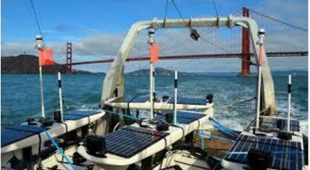
Each vehicle carried identical scientific payloads including a CTD, weather station, wave sensor, and Turner Designs C3 Fluorometer configured with Chlorophyll, Turbidity, and Crude Oil sensors
