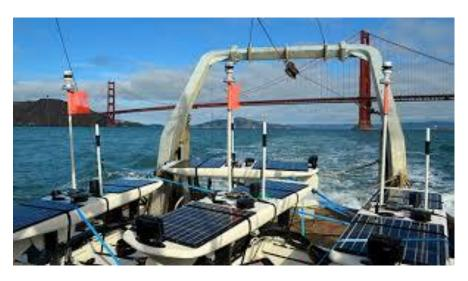
Each vehicle carried identical scientific payloads including a CTD, weather station, wave sensor, and Turner Designs C3 Fluorometer configured with Chlorophyll, Turbidity, and Crude Oil sensors
