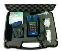
Rapid test methods using fluorometry techniques provide indicative results of algae in ballast waters in less than a minute and are of high interest for rapid compliance testing of ballast water to the D2 standard.
