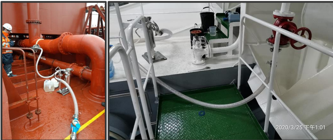
Figure 4. Use of the sampling equipment (BWS1) with a ballast water management system installed on deck (left) and inside an engine room (right).
