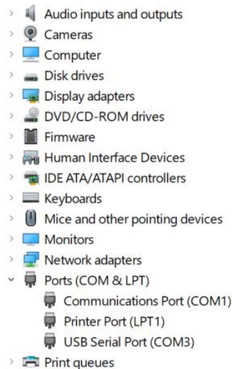
Example image of device manager: CyanoFluor is on USB Port (#3)
