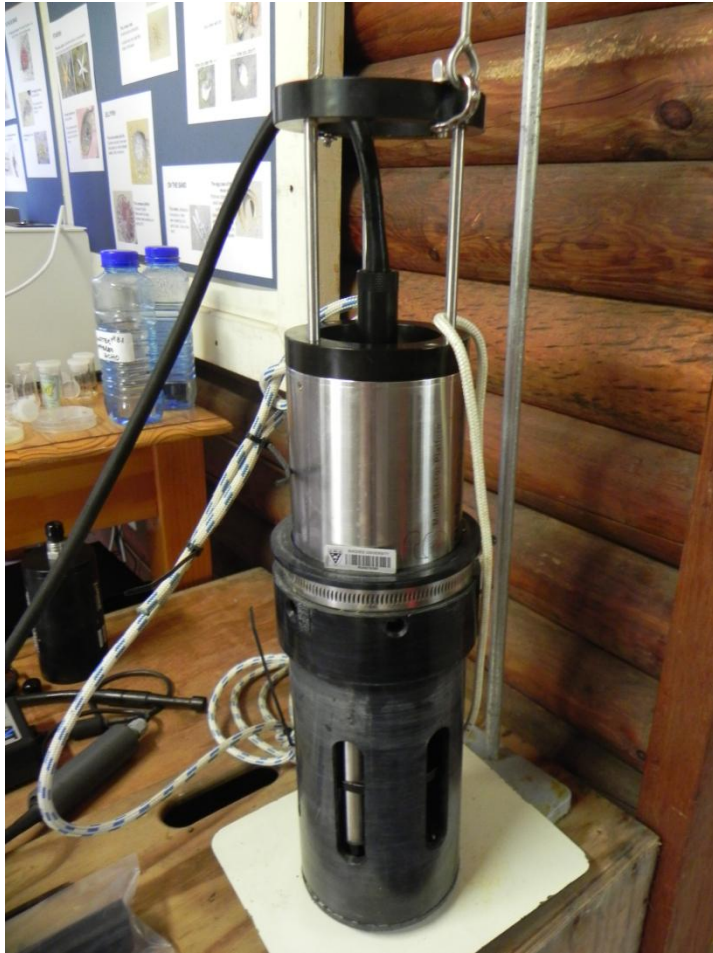
Figure 2. Turner submersible fluorometer: left hand downloading data mode; right had submersible mode with battery pack in place.
