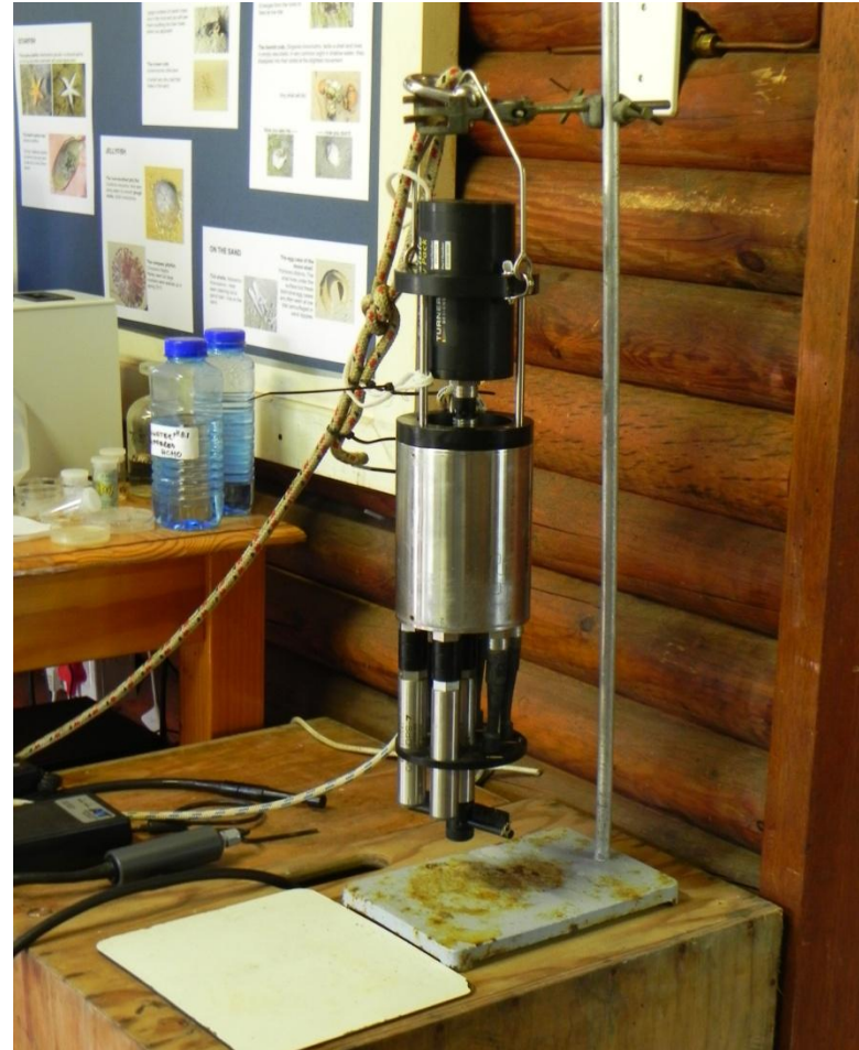
Figure 2. Turner submersible fluorometer: left hand downloading data mode; right had submersible mode with battery pack in place.
